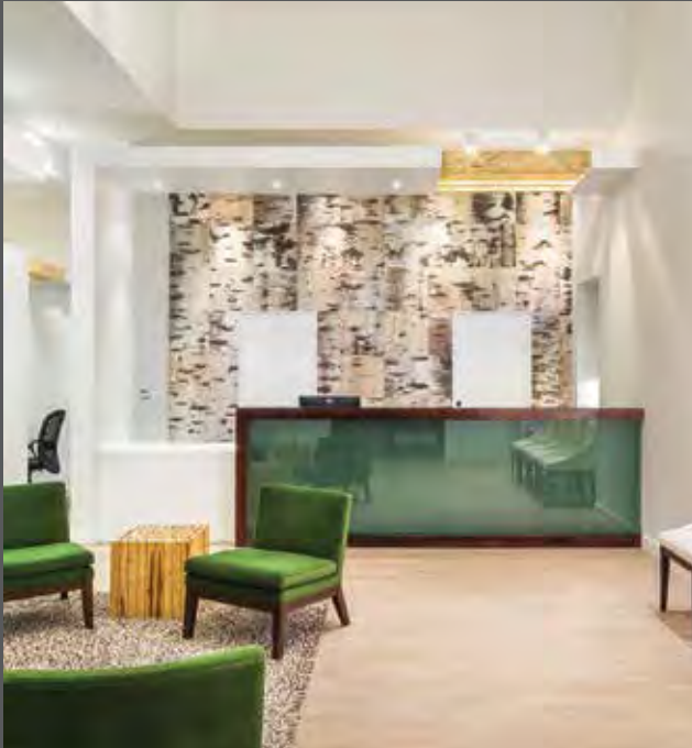
Bark veneer laminates are harvested from living trees using an unrolling process. The resulting veneer can be used as a unique wall covering, as seen behind the reception desk.
